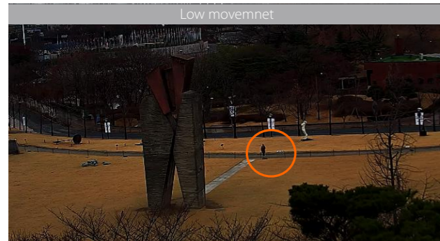
WiseStream II OFF : 7160kbps WiseStream II ON : 74kbps
