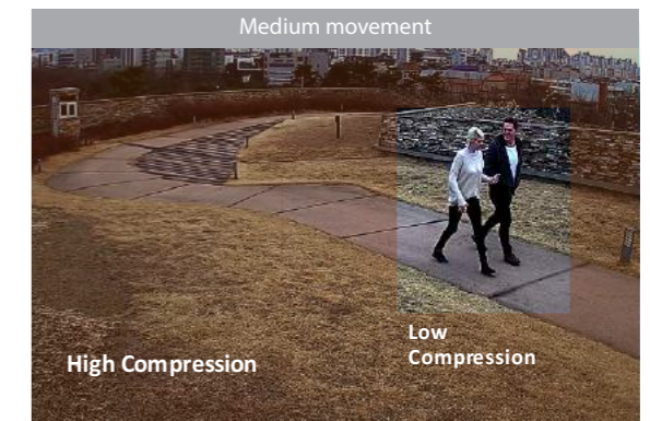
WiseStream II OFF : 7260kbps WiseStream II ON : 1817kbps
