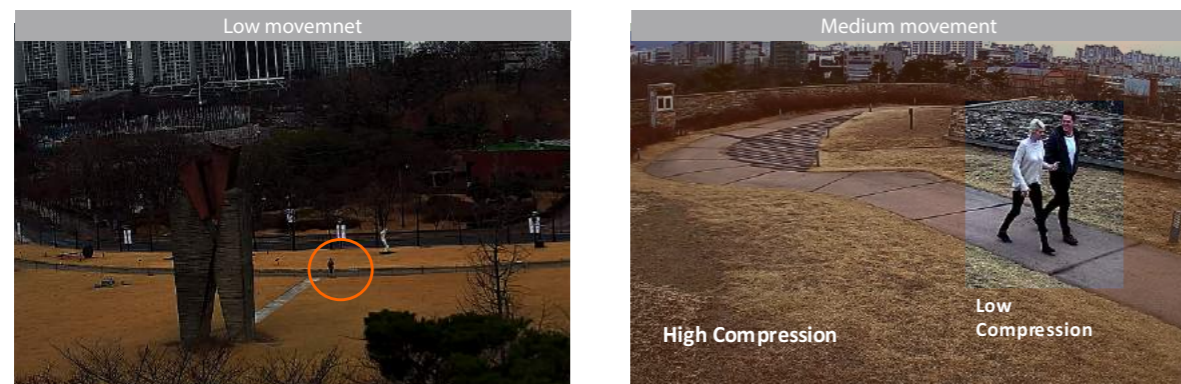
WiseStream II OFF : 7160kbps WiseStream II ON : 74kbps
