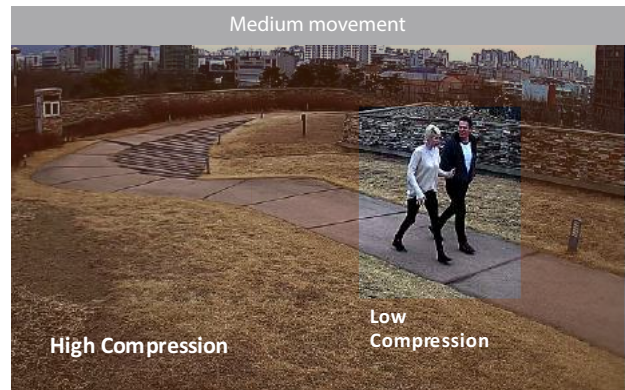
WiseStream II OFF : 7434kbps WiseStream II ON : 3822kbps
