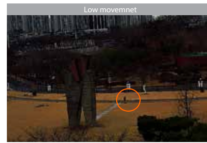
WiseStream II OFF : 7160kbps WiseStream II ON : 74kbps
