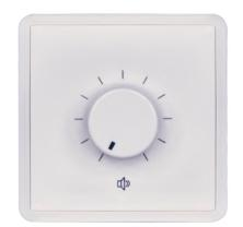
The VC3022 are 100 Volt wall volume controllers with a maximum power handling of 20 Watt, for use in constant voltage public address audio systems.
