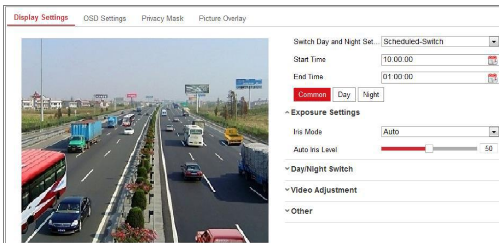
Figure 9-5 Day/Night Scheduled-Switch Configuration Interface
