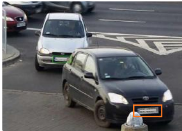
Depth of field is insufficient to cover foreground license plates. Adjust the lens settings.
