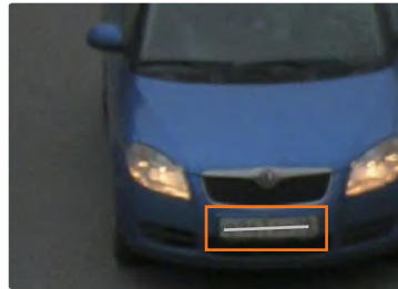
Improper focus settings. Adjust the lens.
