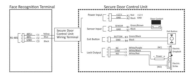
i The secure door control unit should connect to an external power supply separately. The suggested external
