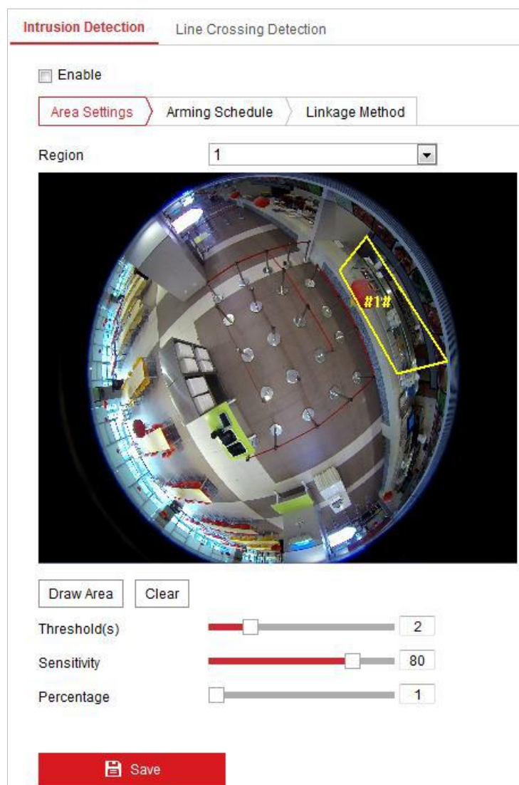
Figure 6-55 Intrusion Detection Settings
