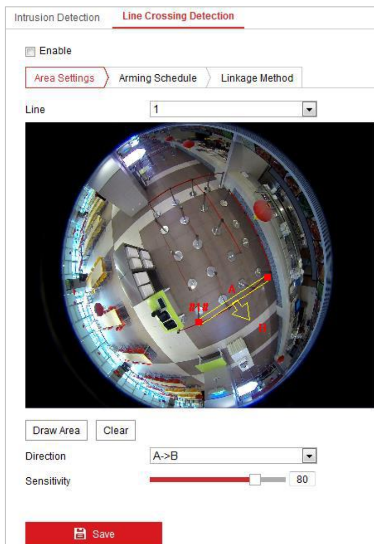
Figure 6-54 Line Crossing Detection Setting
