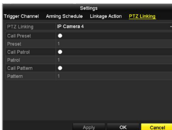
Figure 8-7 Set PTZ Linking of Alarm Input
