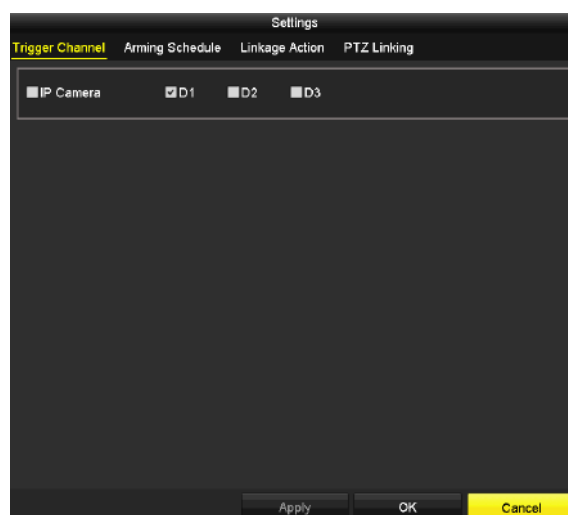
Figure 5-17 Set Trigger Camera of VCA Alarm
