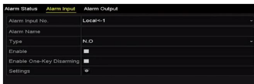
Figure 8-5 Alarm Input Setup Interface
