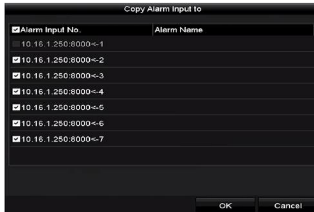
Figure 5-18 Copy Alarm Input
