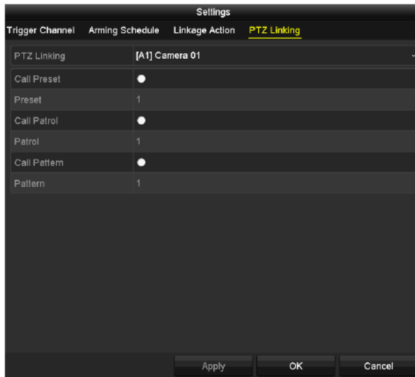
Figure 8-7 Set PTZ Linking of Alarm Input
