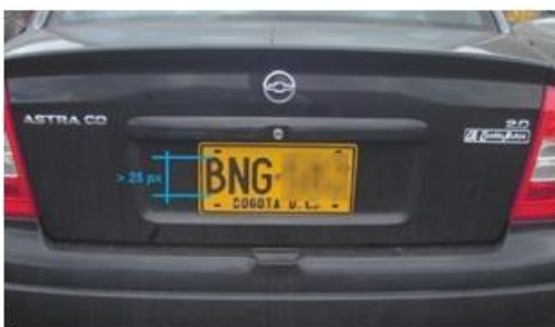
Figure 1, License Plate Pixel Requirement
