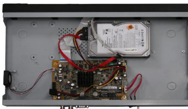
Figure 2-4 Fix Hard Disk
