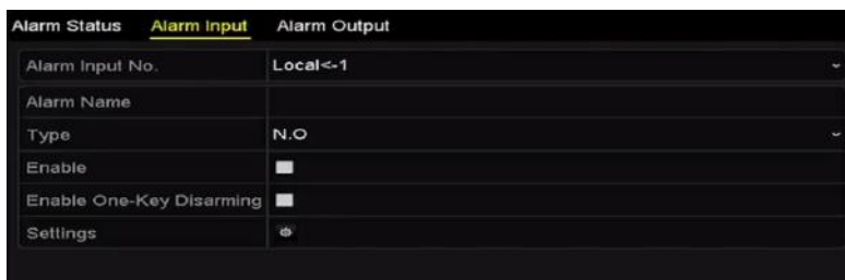
Figure 8-5 Alarm Input Setup Interface
