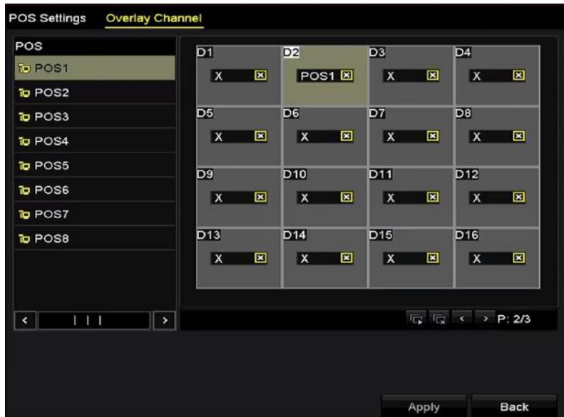
Figure 9-13 Overlay Channel Settings
