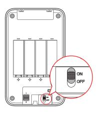
Scan the QR code on the rear panel of the keypad. Push the power switch to ON. Remove the screw on the bottom of the keypad. Disassemble the keypad and remove the rear panel.
