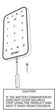
3. Tighten the screw on the bottom to complete the installation.
