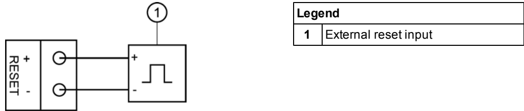
Figure 4-10: Connection for externally resetting the system.
