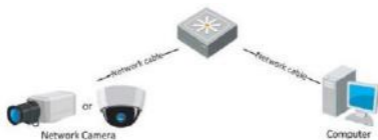
Figure 3-2 Connect via a Switch or a Router
