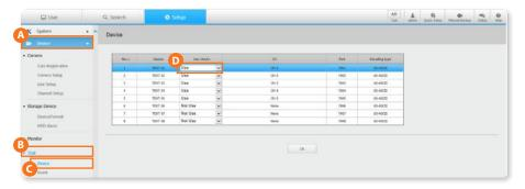
Check the NVR settings to obtain corresponding Port number in (A) Device → B Text → C Device setting (by default port 7001 for CH 1, 7002 for CH 2, etc.)
