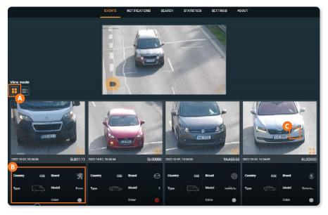
To enable the display of events as a table, click on the (A) corresponding button. In this mode events and their parameters (Date/Time, Plate, Direction, Photo, Country, Type, Brand, Model и Color) are displayed in blocks.
