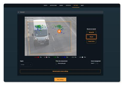
**A Wizard** tool displays the statistic of the latest 1000 recognized plates sizes.
