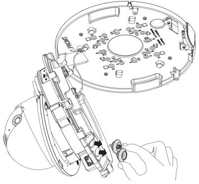
13-1 • Installing network/power cables
