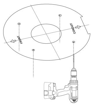
Directly installing on wall/ceiling
