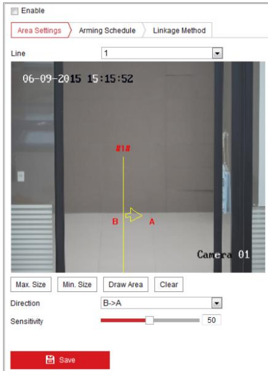
Figure 10-19 Line Crossing Detection
