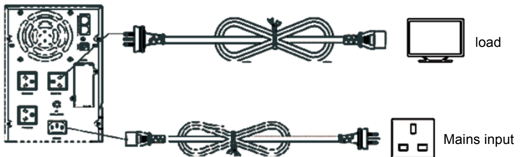
Fig. 3.2.2 Tower 500VA - 2KVA input/output connection diagram
