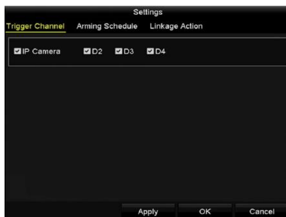
Figure 5-18 Set Trigger Camera of VCA Alarm
