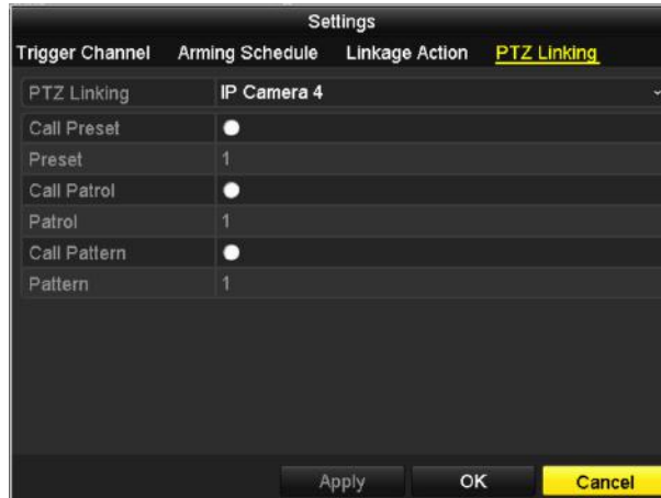
Figure 8-7 Set PTZ Linking of Alarm Input
