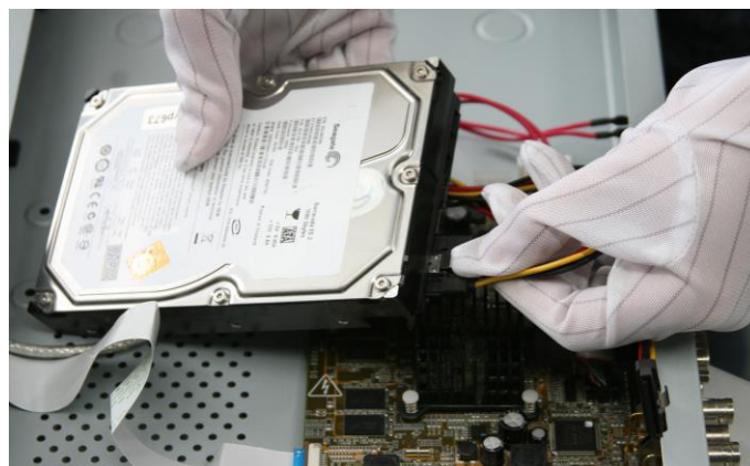
Figure 2. 8 Connect Power Cable
