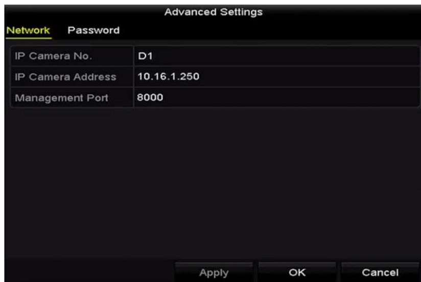
Figure 2-36 Network Configuration of the Camera
