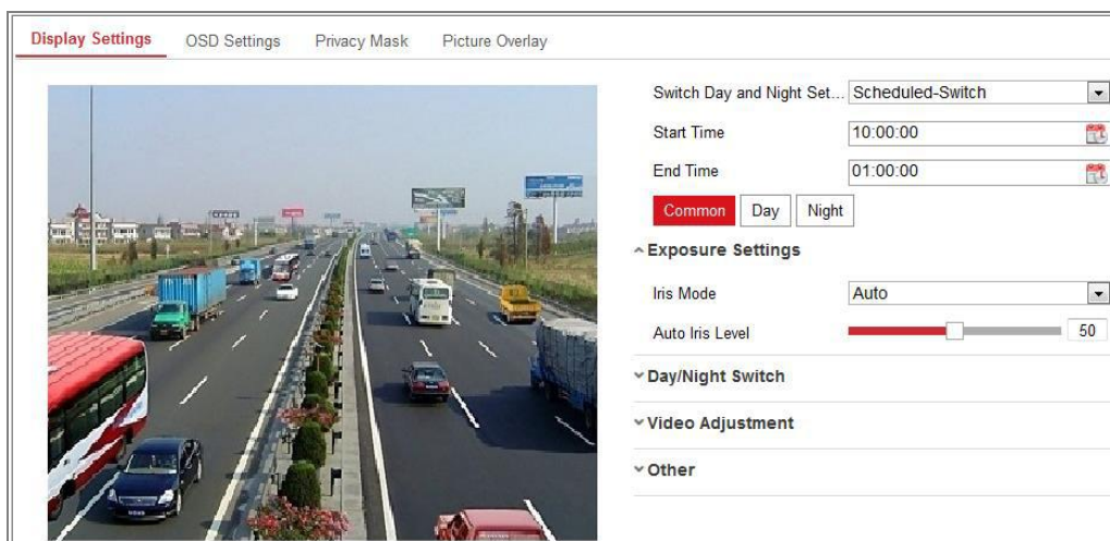
Figure 7-5 Day/Night Scheduled-Switch Configuration Interface
